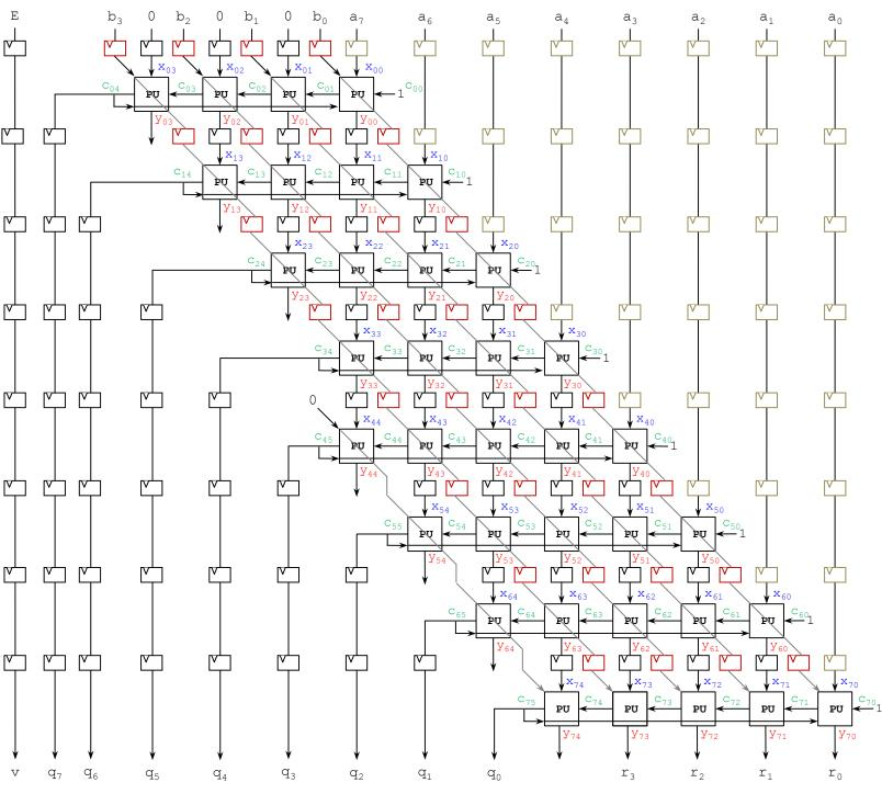
Fully Pipelined Array Divider architecture for N=8, M=4
