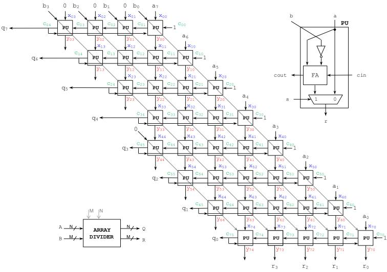
Fully Combinatorial Array Divider architecture for N=8, M=4
